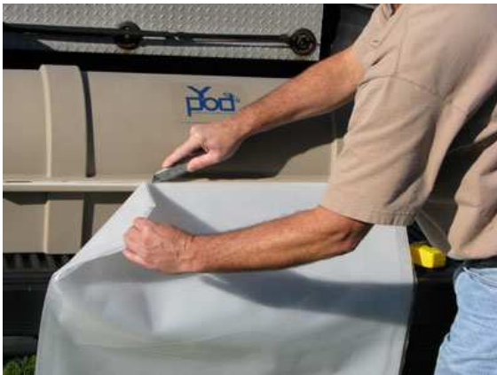
3. Using a utility knife, cut the dispensed material along the cutting guide.
